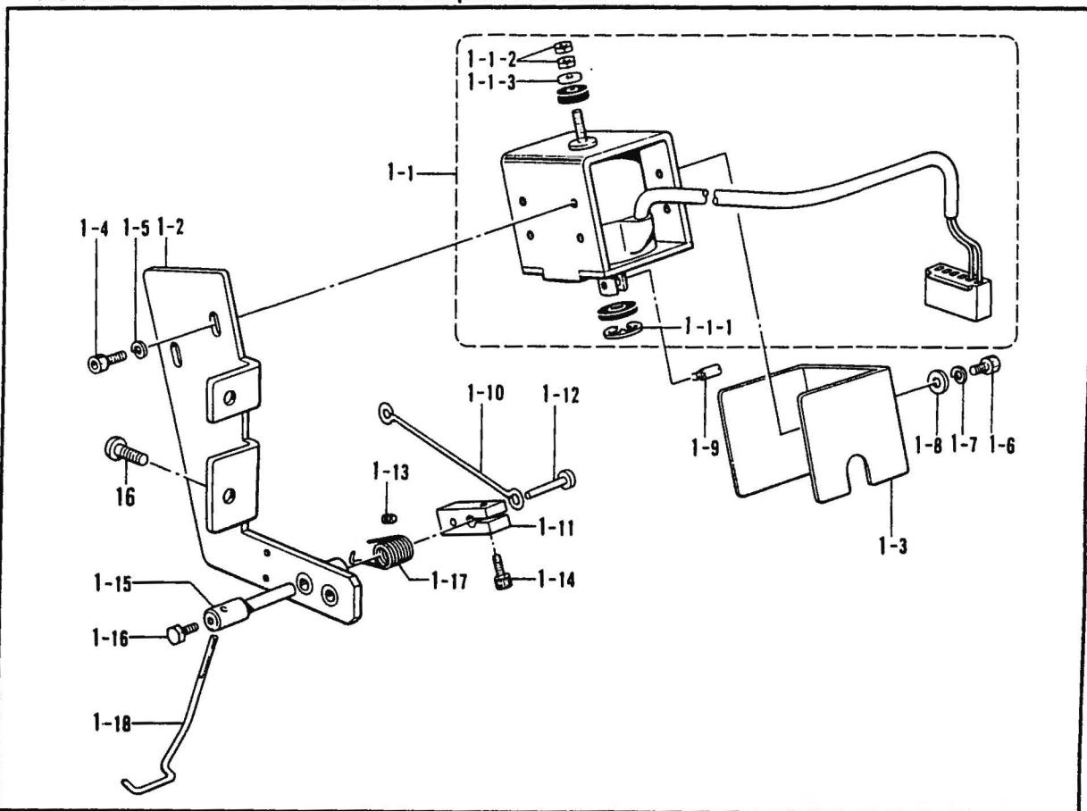
K. 糸サバキ関係/Loop spreading mechanism/Schleifenzieher/Etirement de boucle/Ensanche de bucle
