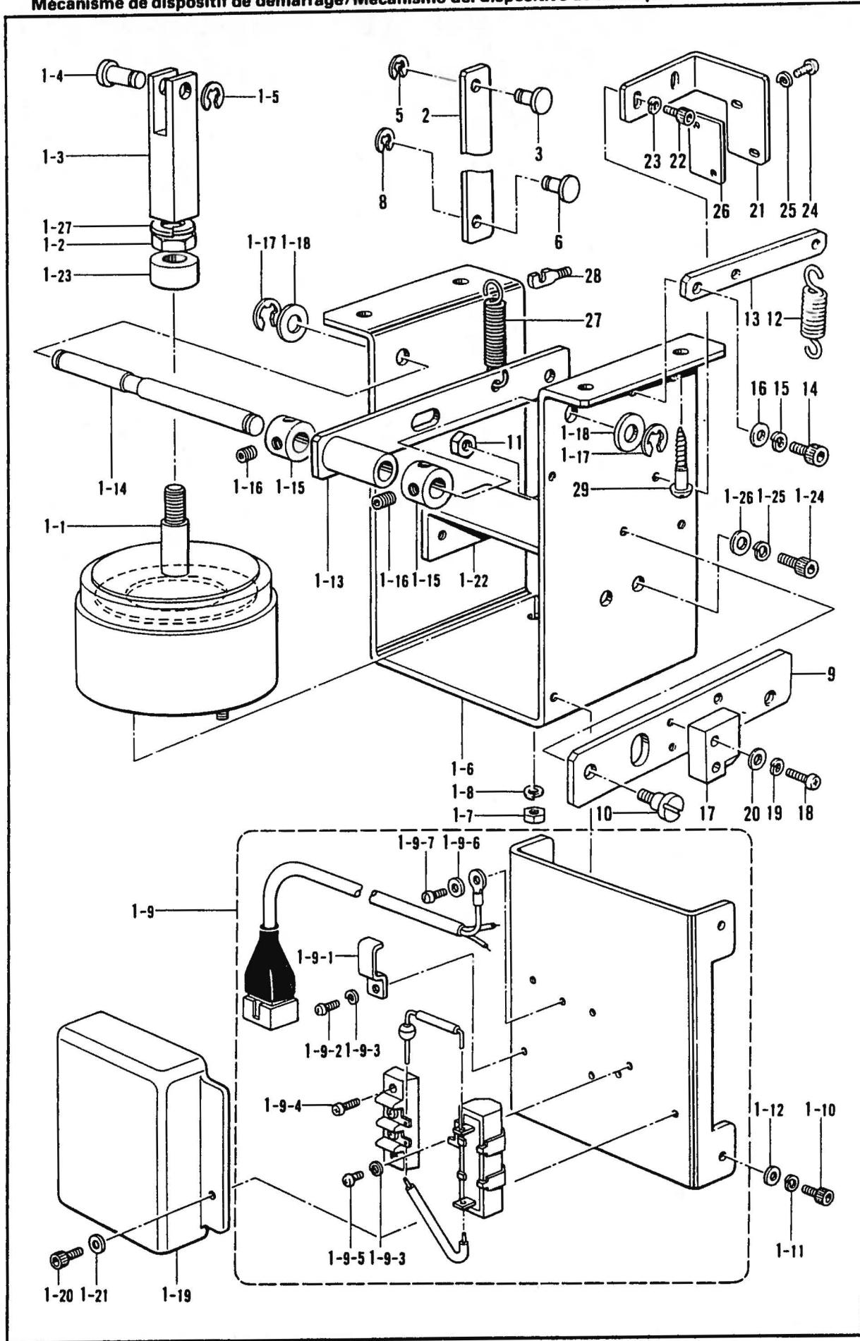
N. 起動装置関係/Starting device mechanism/Startvorrichtung/
