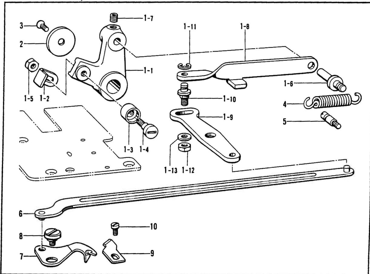
**G. 下軸関係/Lower shaft mechanism/Untere Welle/
