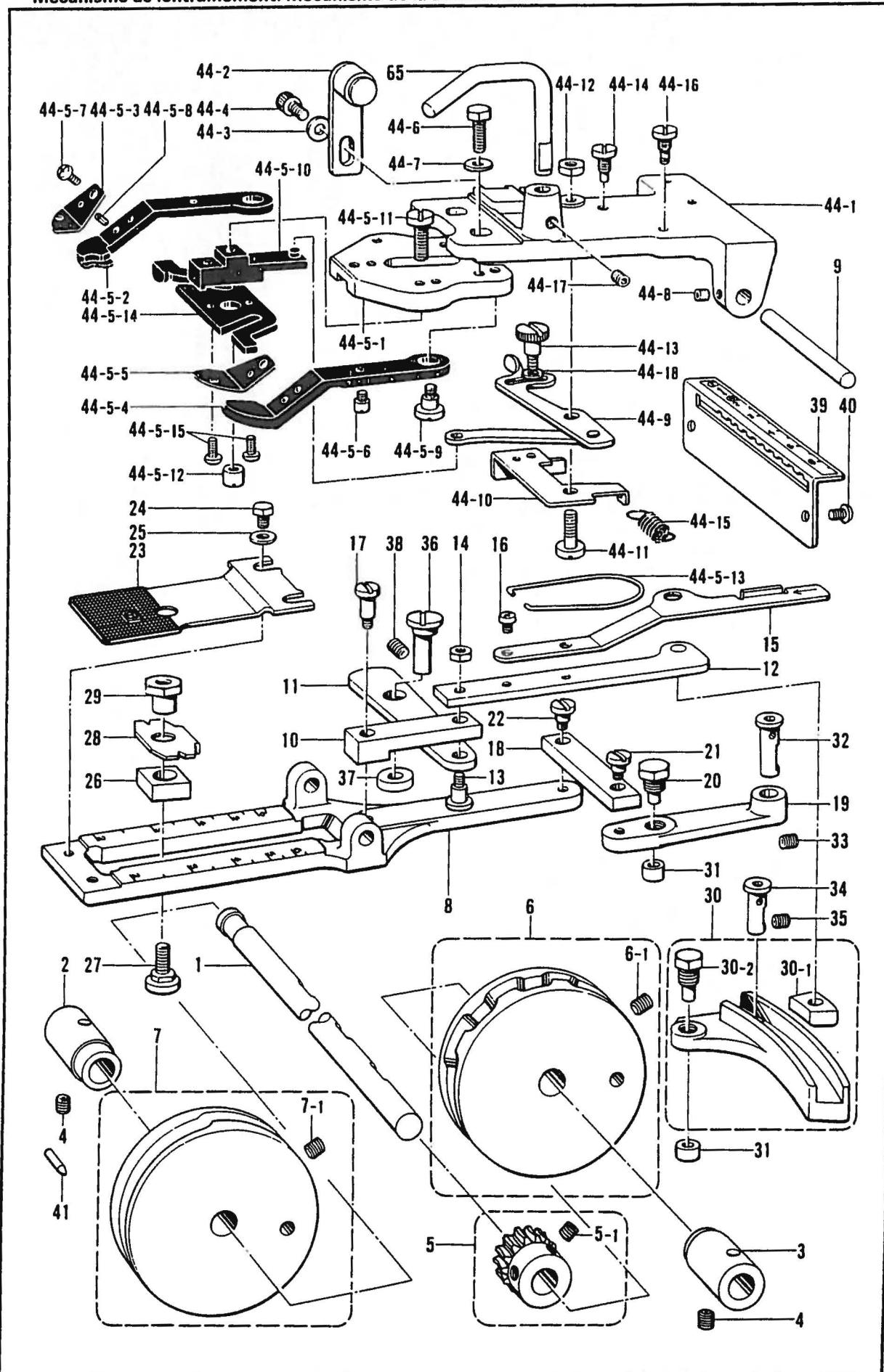
E. 送り関係/Feed mechanism/Transportvorrichtung/
